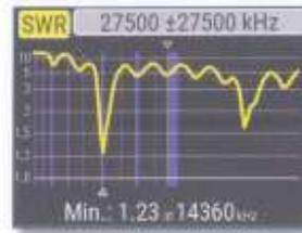
Once your antenna is connected to the analyzer, it is time to measure its characteristics. Press the **4** (SWR chart) key to open the SWR chart screen, then press **OK** to start a new measurement.
